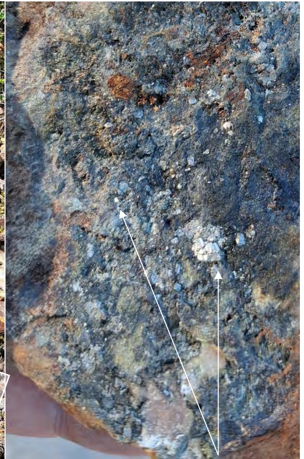
Disseminated fine and coarse-grained arsenopyrite (silver in colour); grab sample location indicated with wide arrow
